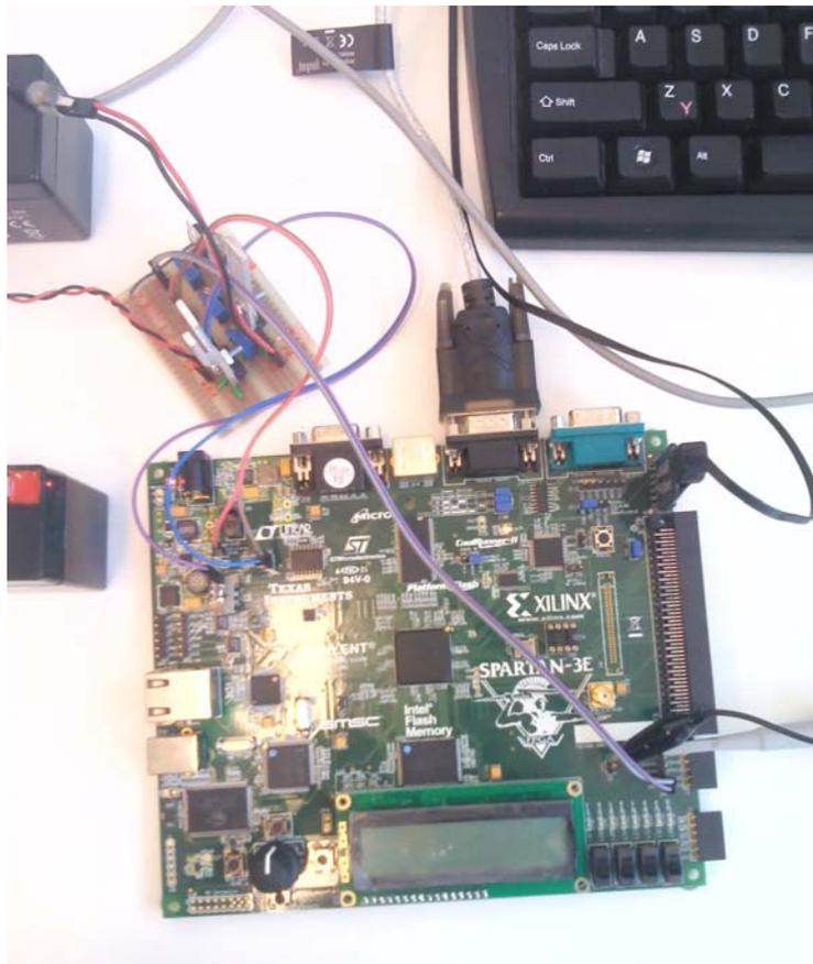
Figure 5.6: FPGA board powered by accumulators, which are connected through stabilizers
